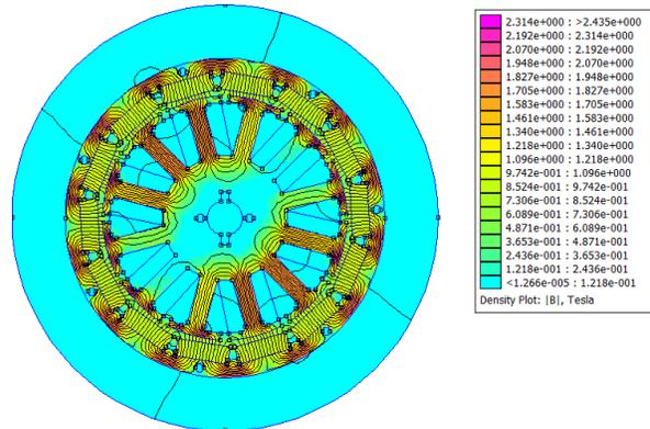
Figure 5: FEMM simulation output for the 60 turn per phase motor at 20A.
