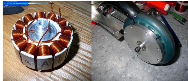
**Figure 3: A kick-scooter wheel motor built by MIT student Charles Guan.**
