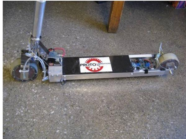
Figure 10: The assembled scooter with two motors installed.
