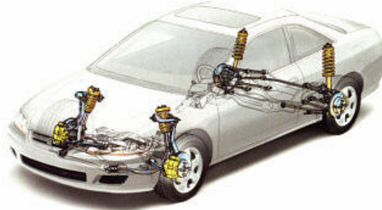
Figure 5: Suspension for a Honda Accord 2005 Coupe.
