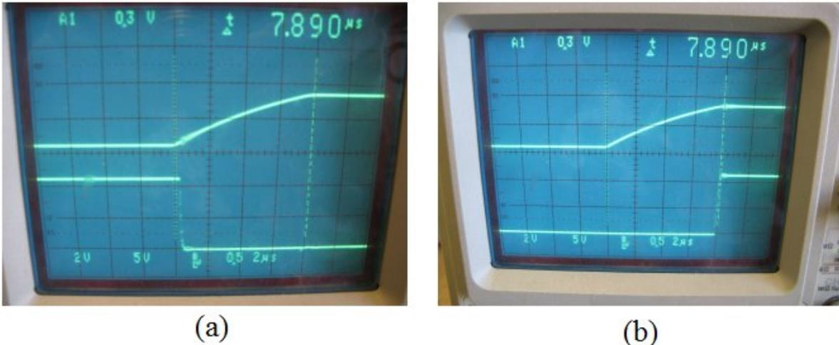
**Figure 9:** The shoot-through protection at work: One MOSFET gate turns off at the start of the transition(a), while the other MOSFET does not turn on until the end of the transition (b). The capacitor sets the duration of the transition, in this case a relatively large  $8\mu s$ .
