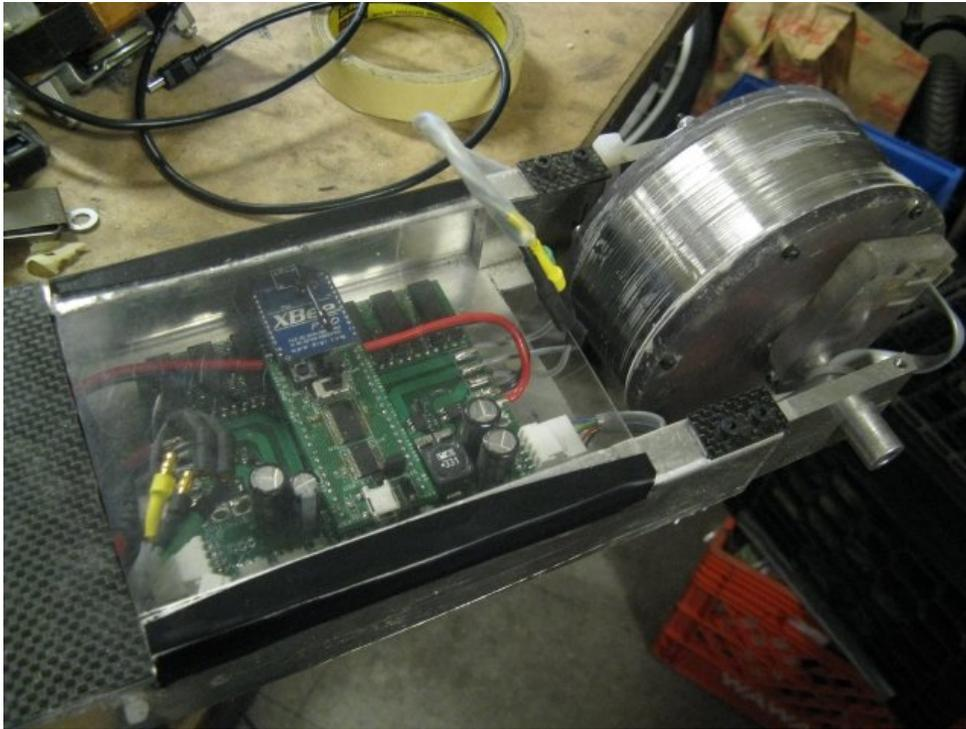
**Figure 16:** The v2.1 controller fits under a transparent cover flush with the scooter deck, so it does not occupy foot space. It is heat sunk directly to the aluminum chassis.
