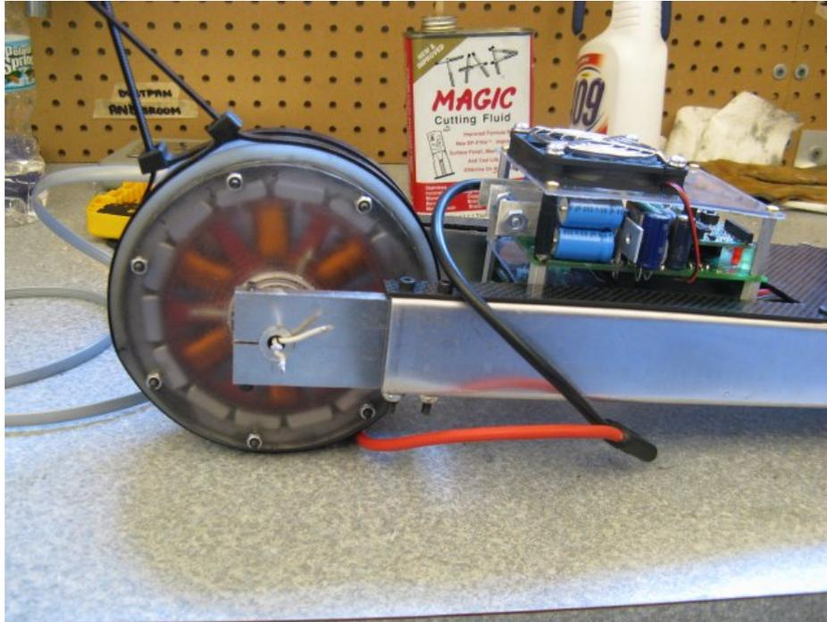
**Figure 14:** The v1.0 controller was for a single motor, so a stack of two was required on the scooter. The stacked controllers took up foot space.
